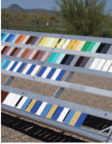
Corus weathering site, Arizona (desert).
